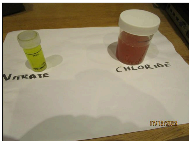
3.1 Item 1(Picture) No salts - Kitchen wall
