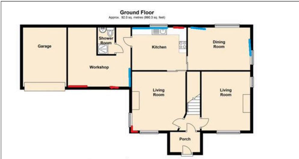
3.0 Item 9(Picture) Ground floor main damp areas
