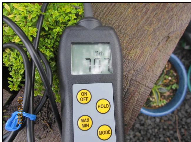
3.2 Item 1(Picture) Hygrometer used externally
